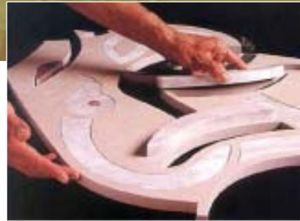
Assembling the waterjet-cut pieces didn’t prove too difficult because of the precise cuts made by the machine. For ease of handling, everything was mounted on specially-cut backer board. (Photo courtesy of Farrodyne USA Inc.)
