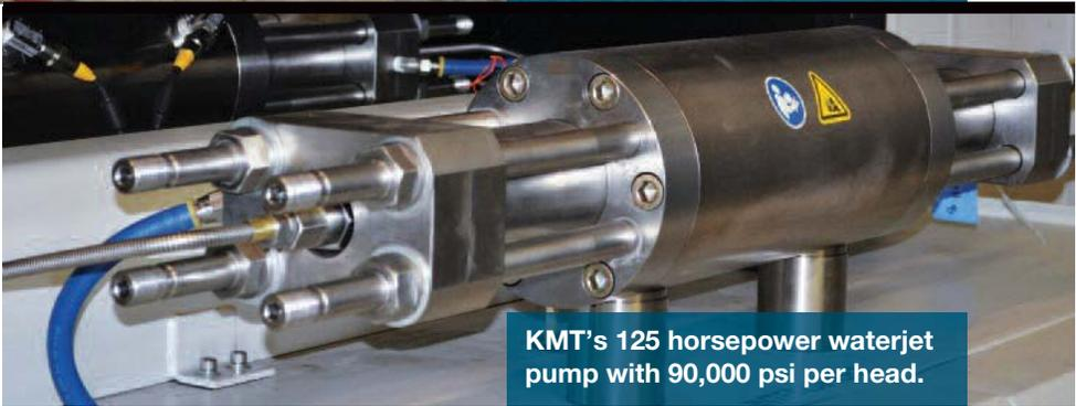
KMT's 125 horsepower waterjet pump with 90,000 psi per head.
