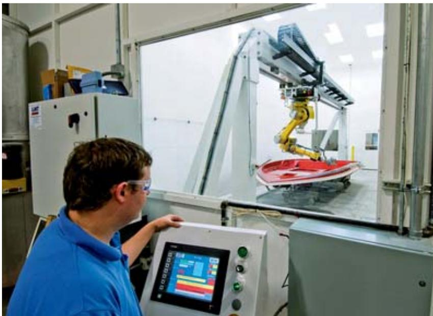
Built by KMT Robotic Solutions, the high-pressure, robotic water jet projects water through a near-microscopic nozzle at 60,000 psi, and according to the company, the process is faster, cleaner and less expensive than man-made cuts.
