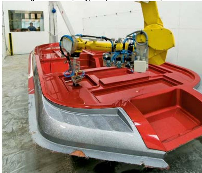
Prior to performing the cuts, the JetTool initiates a calibration process using lasers to measure the precise placement of the cutouts. The unit is able to work on all current Ranger models, being capable of cutting a boat up to 25 feet.
