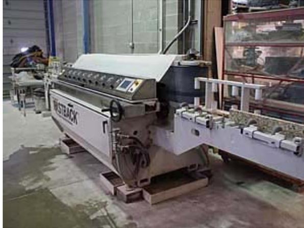
A flat-edge polishing machine is used for polishing the edges of countertops.
