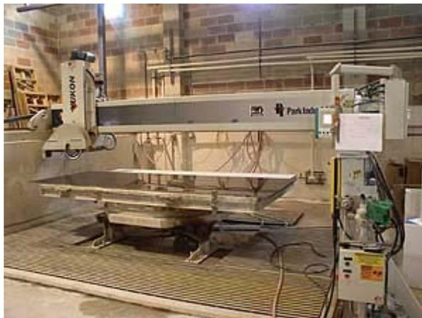
A Yukon bridge saw is utilized to cut slabs during the production process.
