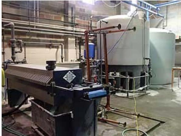
A Hy-Pack water treatment system from Beckart Environmental, Inc. of Kenosha, WI, was put in place four years ago to recycle water used during fabrication.
