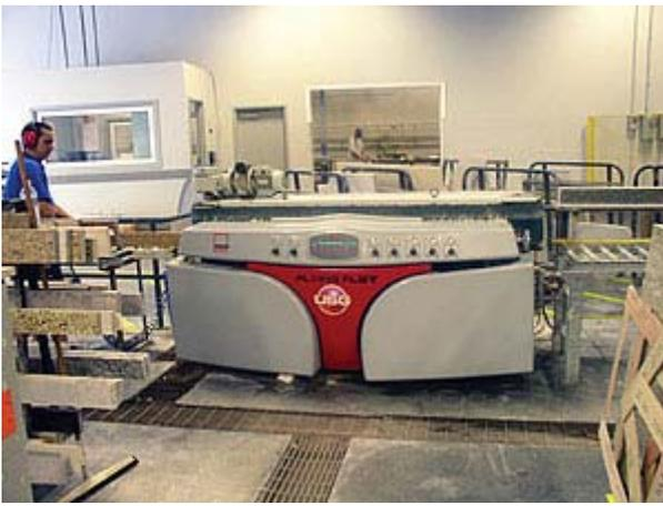
A Flying Flat edging machine from Sassomeccanica is used for processing backsplashes.
