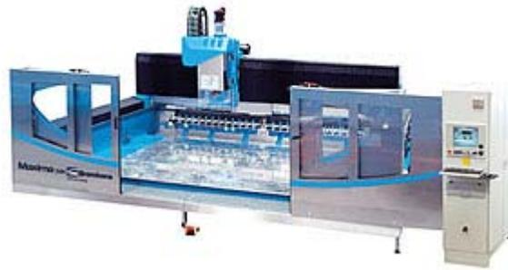
The Ft. Myers and Orlando locations each operate a CMS/Brembana Maxima CNC stoneworking center (an example of which is pictured).
